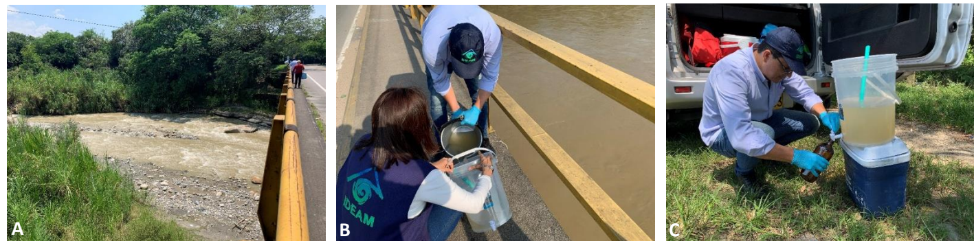
Photo 13. A) Sampling site at the river Paéz, B) grab water sampling, and C) dividing the water sample into subsamples.
